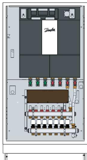
The flat station and the distribution unit fits on the back plate of the recess boxes but can also be mounted on the wall.
