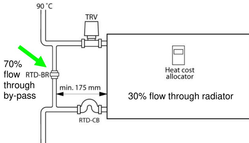
RTD-BR is used in 1-pipe system with TRV and Backflow Restrictor (RTD-CB). RTD-BR is used to insure enough flow through the radiator. RTD-BR will decrease by-pass with one dimension, and thereby secure enough flow through the radiator if flow pipe, return pipe and by-pass pipe is the same dimension. RTD-BR is made in black steel.
