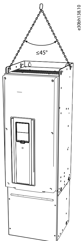
Figure 2: Lifting the Enclosure Sizes MR8 and MR9
