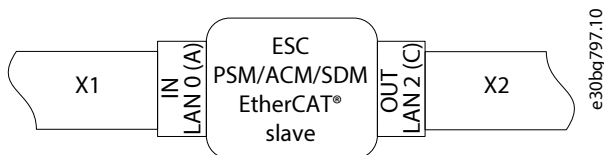
Figure 20: EtherCAT® Port Assignment for the Power Supply Module (PSM 520), Servo Drive Module SDM 521/SDM 522
