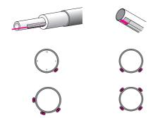
The self-limiting heating cable may only be used for installations with pipes of metal or plastic.
