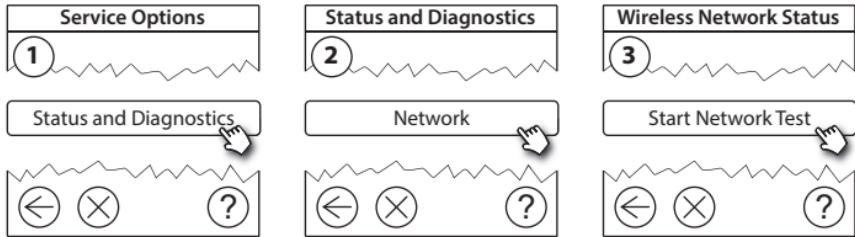
At the end of the network test the Danfoss Link™ CC awaits for all battery operated devices to wake up and report. Follow the instructions given on the screen. If the network test is running smoothly, there will be no need for further interaction. If the network test is performing slow, the Danfoss Link™ CC guides through trouble shooting and gives useful tips for speeding up the process.
