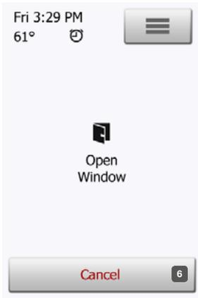
This option allows you to enable the “Open Window” function. The thermostat can detect an open window by registering a rapid drop in temperature.
