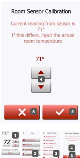
This option allows you to calibrate the room sensor.
