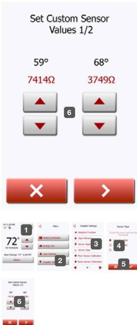
This option allows you to choose the type of floor sensor used with the thermostat. You can thus choose to use an existing sensor with the thermostat, e.g. in renovation projects.
