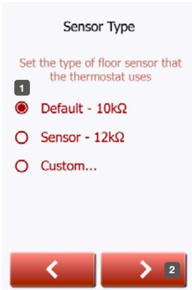
Choose which floor sensor type is used with the thermostat.
