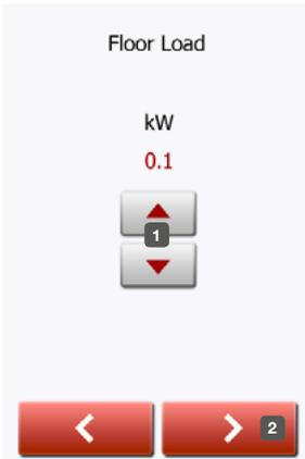
1. Set the load of the underfloor heating system to be controlled by the thermostat.
