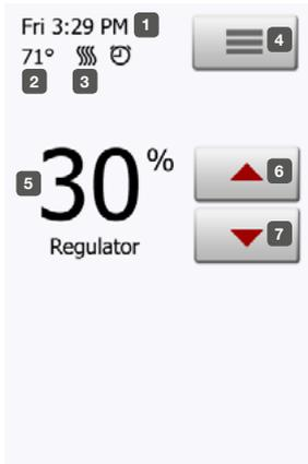
In this mode, the thermostat operates as a regulator and no sensors are used. The setting is a percentage of the full load in steps of 10%. Note that Floor Protection is not active when using the thermostat as a regulator. Regulator mode is activated under **Menu/Installer Settings/Sensor Application/Regulator**
