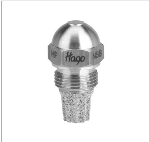
Many nozzles are satisfactory for spraying liquids, but for a positive cut-off ask for the Hago type 4023 nozzle. Our exclusive design produces a precisely controlled flow rate and spray angle and includes a liquid cut-off near the orifice. Fluid cut-off near the orifice can be very important in situations where excessive after drip can damage or destroy things located beneath the nozzle.
