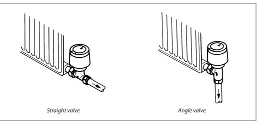
FJVR is mounted in the radiator outlet. The valve and sensor can be fitted in any position as long as flow direction is observed. During construction, the heat can be controlled by turning the slotted screw in the valve cap, prior to fitting the element.
