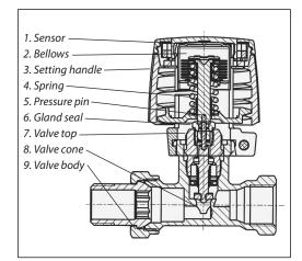
The return temperature limiter includes a thermostatic element type FJVR and a valve body type FJVR 10.
