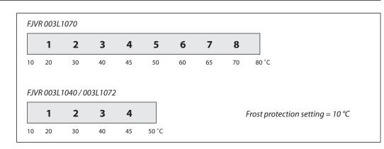
Required return water temperature can be set by turning the dial. The scale figure indications appear as in the il-lustration.
