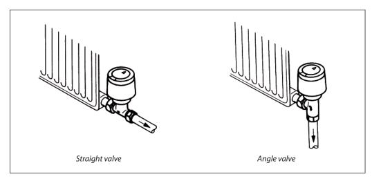
FJVR is mounted in the radiator outlet. The valve and sensor can be fitted in any position as long as flow direction is observed.
