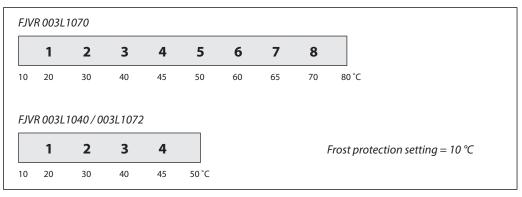
Required return water temperature can be set by turning the dial.
