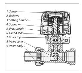
The return temperature limiter includes a thermostatic element type FJVR and a valve body type FJVR 10
