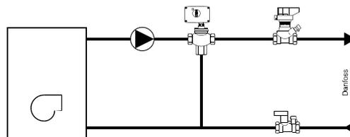
Boiler, flat station or heat pump in 1-family houses.
