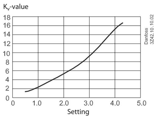
Flow Diagrammes, DN 40 LENO™ MSV-O DN 40
