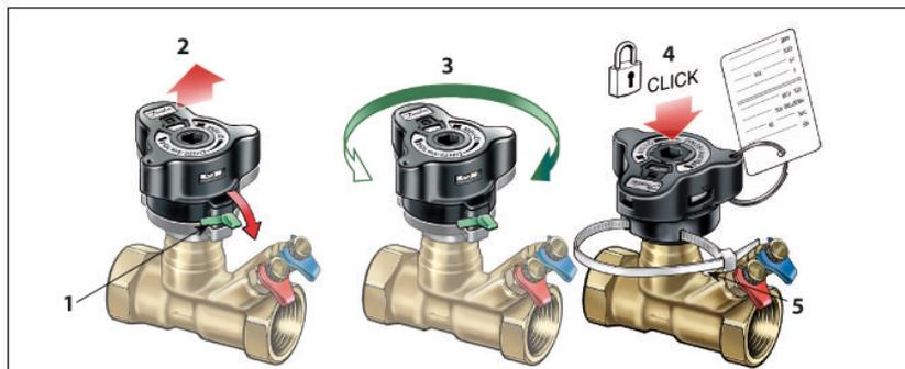
The valve has a built-in presetting feature for accurate flow ratings.
