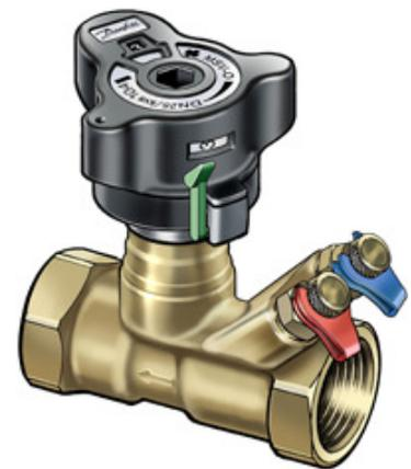
It is recommended to use LENO™ MSV-O in constant flow systems in front of boilers, flat stations or heat pumps in one-family houses for balancing, shut-off function for service and repair, flow verification, one pipe systems. The valve may be mounted in flow or return.
