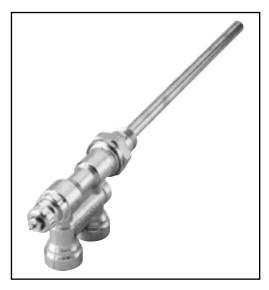
The RA 15/6T and TB is a special conversion valve that allows a single connection point-at the side of the radiator- to serve as both the supply & return for a hot water based system. An example of its application is the transformation of a 1-pipe steam system into a hot water based system.
