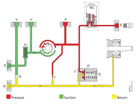
From the suction inlet (S) oil is drawn through the filter (H) to the gear set, where the pressure is increased. When voltage is applied to the NC-valve, it opens and releases oil to the nozzle outlet.
