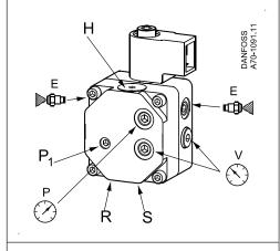
S: Suction inlet G1/4 Return outlet G1/4 R: E: Nozzle outlet G 1/8 P: Pressure gauge port G 1/8 V: Vacuum gauge port G 1/8
