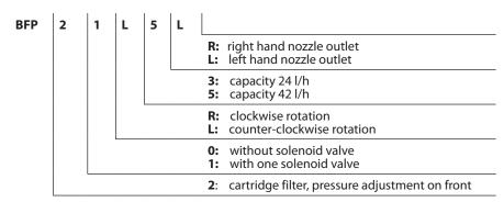
Nozzle capacity at 4.3 cSt., 10 bar, 2800 min-1
