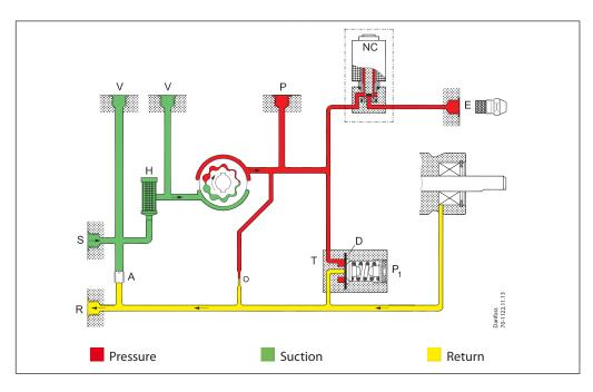
From the suction inlet (S) oil is drawn through the filter (H) to the gear set, where the pressure is increased. When voltage is applied to the NC-valve, it opens and releases oil to the nozzle outlet.
