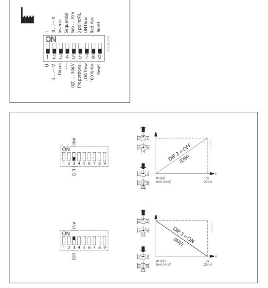
The actuator has a selection of DIP switches under the removable cover. The switch provides the following functions:
