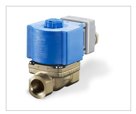
EV260B is a proportional (modulating) servo-operated 2-way solenoid valve with connections from 1/4" to 3/4".
