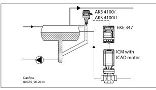
System configuration ICAD Regulating principle: Low Level Signal setup: AKS 4100/U
