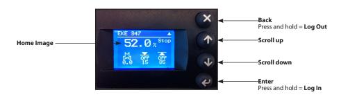
The user interface of the control panel consists of a multiline display and 4 individual push buttons: Enter button, Scroll up button, Scroll down button and Back button. The figure shows the Home display image, which give the actual overview. This is the starting point for entering into menus, and you will revert to this image by pushing B 1 – 3 times (depending on actual position).
