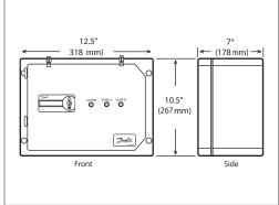
The GX 850 Dual Zone Automatic Control Panel (ACP) is the most optimal solution for keeping an area free of ice and snow. The GX 850 acts on information received form sensor(s) which register both temperature and moisture, then calculates the information ensuring that the heat will only be turned on when snow and/or ice is present. The result is optimal performance with maximum energy savings and minimum operating costs.
