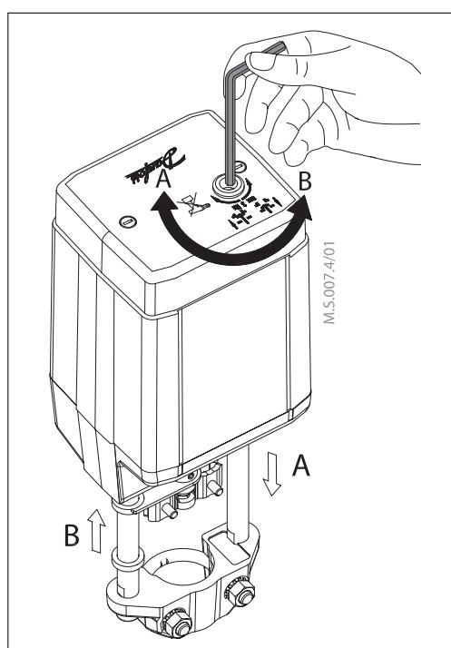
The manual override is applied by rotating the 4 mm Allen key (not supplied) to the required position. Observe the direction of the rotation symbol.
