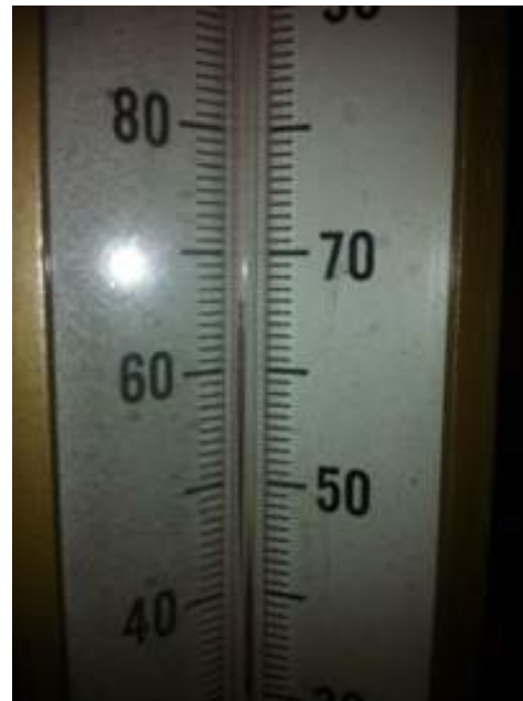
After PICV = 64° F return water temperature (63% improvement)
