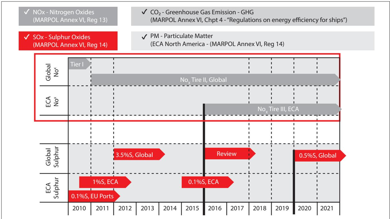
Figure 2: Overview of IMO requirements to emissions from vessels. Source: IMO
