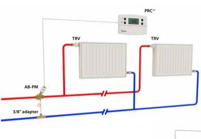
AB-PM: Pressure differential controller with flow
