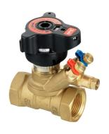
In the supply pipe mounted shut-off partner valves are used to measure the differential pressure by a capillary tube connected to both valves. ASV-P and ASV-PV can be connected to ASV-M, ASV-I or ASV-BD partner valves. Flanged ASV-PV can be connected to MSV-F2 partner valves. Some partner valves can also be used for manual limitation of the maximum system flow.
