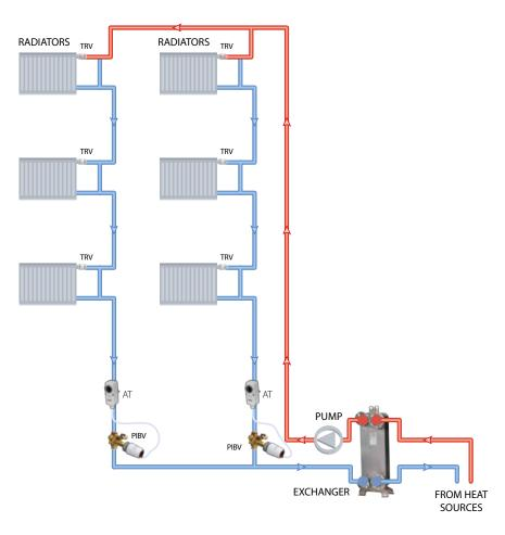
TRV – Thermostatic Radiator Valves PIBV – Pressure Independent Balancing Valves (as flow limiter) AT – Pipe Thermostat
