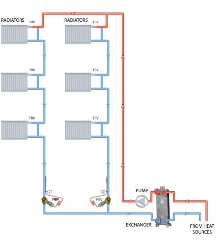
TRV – Thermostatic Radiator Valves PIBV – Pressure Independent Balancing Valves (as flow limiter) QT – Self Acting Thermostat
