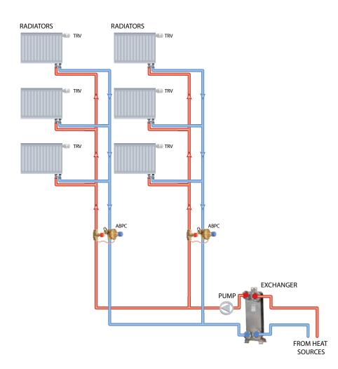
TRV – Thermostatic Radiator Valves ABPC – Automatic Balancing Pressure Controller
