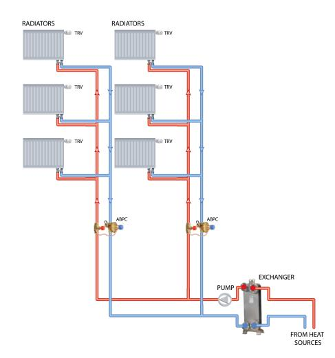
TRV – Thermostatic Radiator Valves ABPC – Automatic Balancing Pressure Controller
