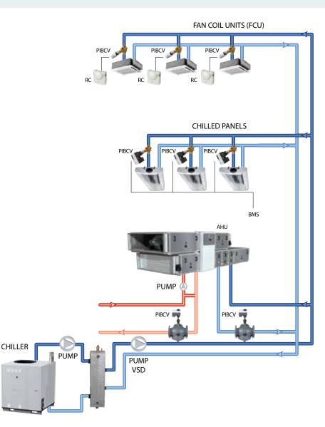
PIBCV – Pressure Independent Balancing Control Valves (as a flow limiter) RC – Room Controller BMS – Building Management System VSD – Variable Speed Drive
