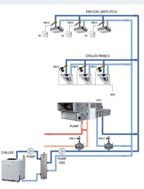
PIBCV – Pressure Independent Balancing Control Valves RC – Room Controller BMS – Building Management System VSD – Variable Speed Drive
