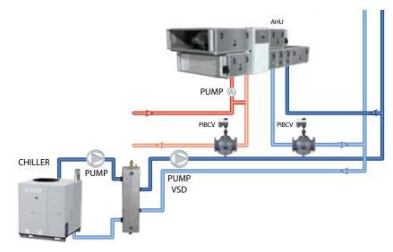
**PIBCV** – Pressure Independent Balancing Control Valve **AHU** – Air Handling Unit
