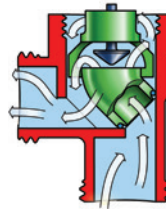
Revolver mechanism correcting water flow within valve in situations of reverse flow.
