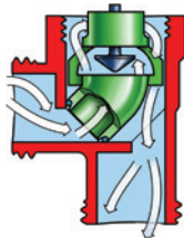
Water flowing correctly through the Revolver Valve, whilst set in factory set position.
