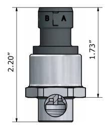
Shown with Packard Metri-Pack and SAE female flare with depression pin. Please contact Danfoss for other available configurations.
