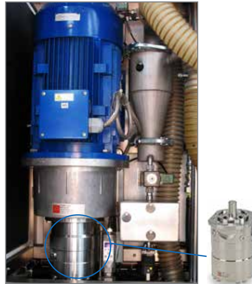
The Danfoss PAHT high-pressure pump is a part of the cleaning system manufactured by SLE Technology
