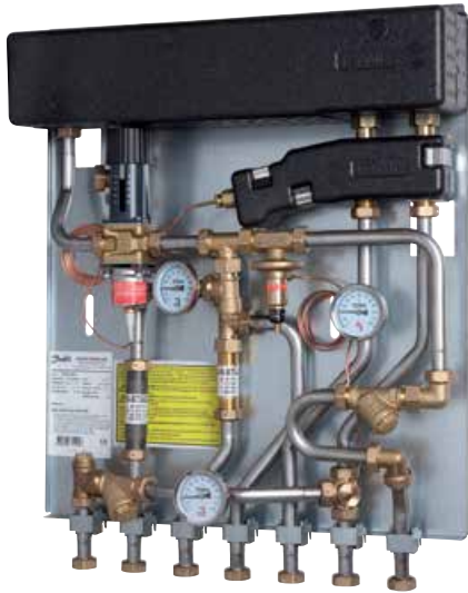
Danfoss series Termix VMTD-F flat stations are complete hydronic interfaces with a compact but powerful plate heat exchanger that provides hot water immediately when the tap is opened. The station can also be supplied with connections for space heating, including fittings for controlling radiators or floor heating systems.
