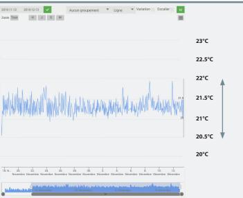
The temperature fluctuates by  $\pm -0.5$ °C from the actual temperature.
