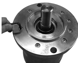
10. Screw the 8 screws into the flange and the housing.
