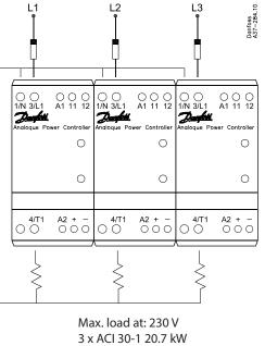
3 x ACI 30-1 20.7 kW 3 x ACI 50-1 34.5 kW Three phase with single-phase contactor ECI-1 as slave Only burst firing mode
