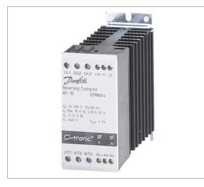
RCI reversing contactors are designed for demanding forward/reverse control of three-phase AC motors. The zero cross switching method ensures very fast and precise motor control and virtually eliminates EMC emission. The RCI reversing contactor is ideal where fast switching capability and long life are essential. Typical applications are conveyors, thread cutting machines, packaging lines and other applications where fast reversing capabilities are needed.
