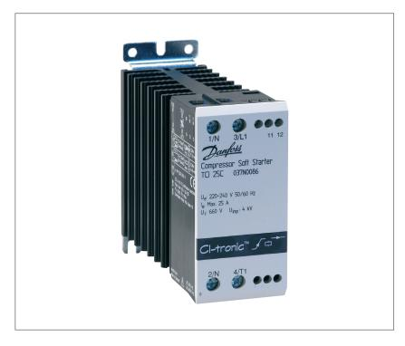
The TCI 25C soft starter is designed for soft starting of single-phase compressors. During start the TCI 25C will gradually ramp-up the motor voltage to full line voltage thus reducing the starting current peak.
