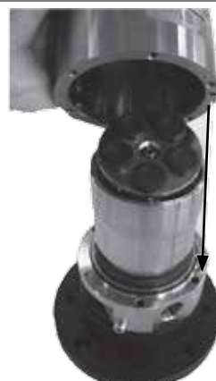
20. Position the housing on the port flange and over the guide pin.
