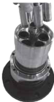
19. Position the new spring, new spring guide, new retainer guide, new retainer plate and new pistons.
