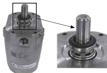
22. Mount the new shaft seal following the instructions on the next pages.
