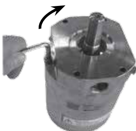
21. Hold the pump together and carefully turn it over to rest on the housing. To prevent seizing-up, lubricate the threads on the 4 screws and screw them into the port flange and the housing. Use Molykote D paste from Dow Corning or Klüber UH1 84-201 from Klüber Lubrication. Tighten the 2 flange screws to a torque according to exploded view.
