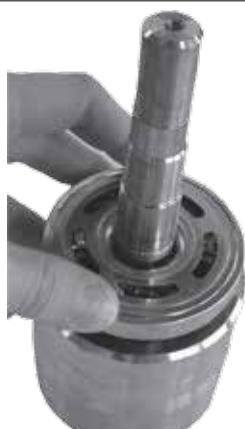
11. Gently press, by hand, the valve onto the cylinder barrel.
