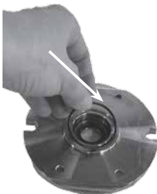
23. Replace the O-ring on the SAE flange.
