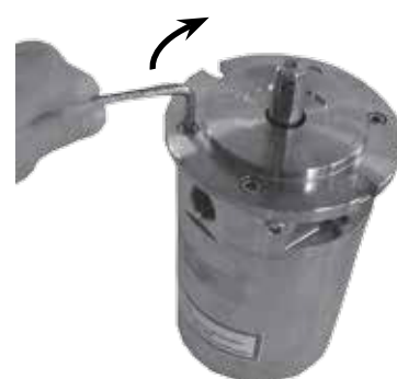
24. Lubricate the threads on the 4 screws with grease and screw them into the pump and tighten by hand. Use Molykote D paste from Dow Corning or Klüber UH1 84-201 from Klüber Lubrication.
