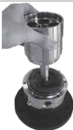
7. Remove the cylinder barrel.
