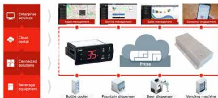
Figure 2. Danfoss Prosa IoT solutions: a complete service, from heterogeneous Equipment to Enterprise processes.
