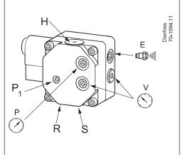
P<sub>1</sub>: Pressure adjustmentS: Suction inlet G 1/4
