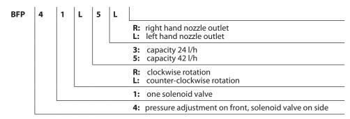
Nozzle capacity at 4.3 cSt., 10 bar, 2800 min-1
