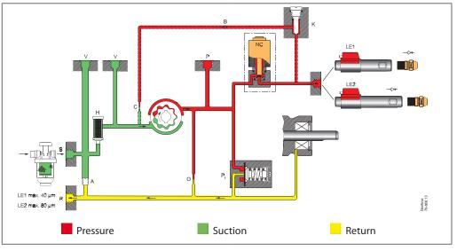
The LE pump is used with either an LE nozzle (System 1) or an LE preheater (System 2). Before burner start the preheater heats up the oil in the nozzle line. The expanding oil is prevented from dripping out of the nozzle because of the connection back to the suction side. The non return valve B inside the pump has an opening pressure of less than 2 bar whereas the LE valve in the nozzle opens at a pressure of  $5\pm 1$  bar. (The valve in the preheater opens at min. 6 bar.)
