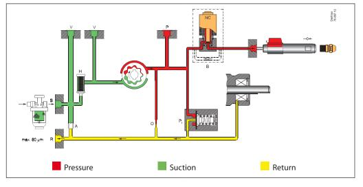
Before the burner starts the oil is heated in the oil preheater and in the nozzle line. This causes the oil to expand. The safety shut-off valve in the preheater prevents the oil from dripping out of the nozzle because the check valve B in the solenoid valve opens and thus makes a connection to the return or suction side of the pump.
