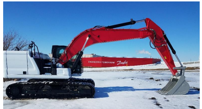
Figure 2: Danfoss Digital Displacement Excavator
