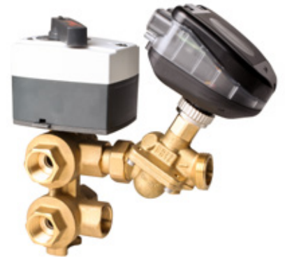
Danfoss NovoCon®, mounted on AB-QM, controls both the flow through the PICV valve and the position of the CO 6 actuator mounted on the heating/cooling 6-way ChangeOver valve.
