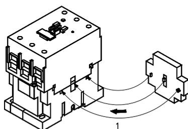
Mechanical interlocks are used in reversing systems, automatic transfer switching equipment (ATSE) or star-delta systems.
