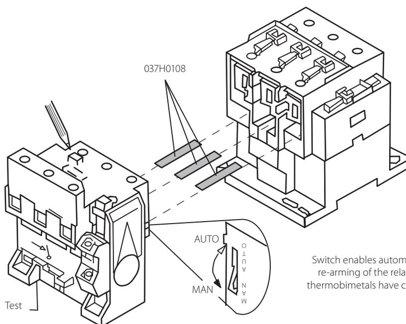
Test allows checking the functioning of signal circuits.
