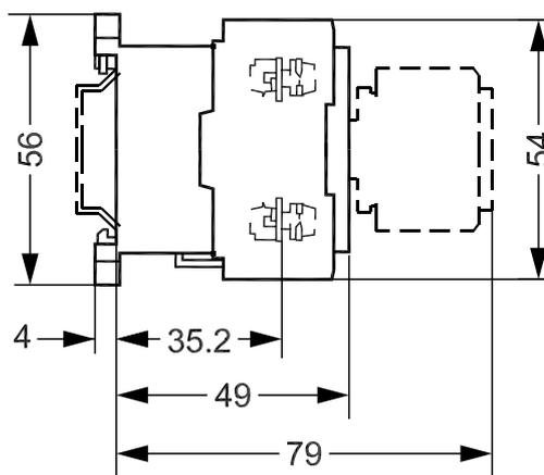
Dimensional drawing of the mini-contactor set with thermal overload relay
