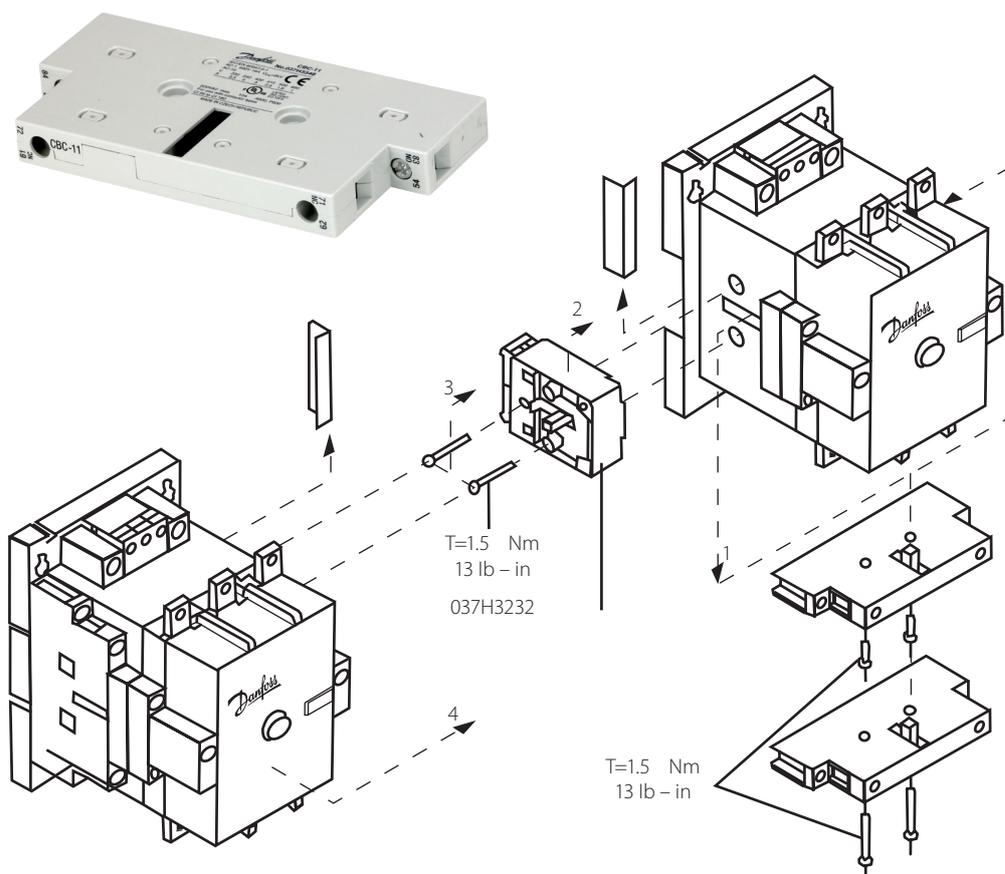
Mechanical interlocks are used in reversing systems, automatic transfer switching equipment (ATSE), or star-delta systems.
