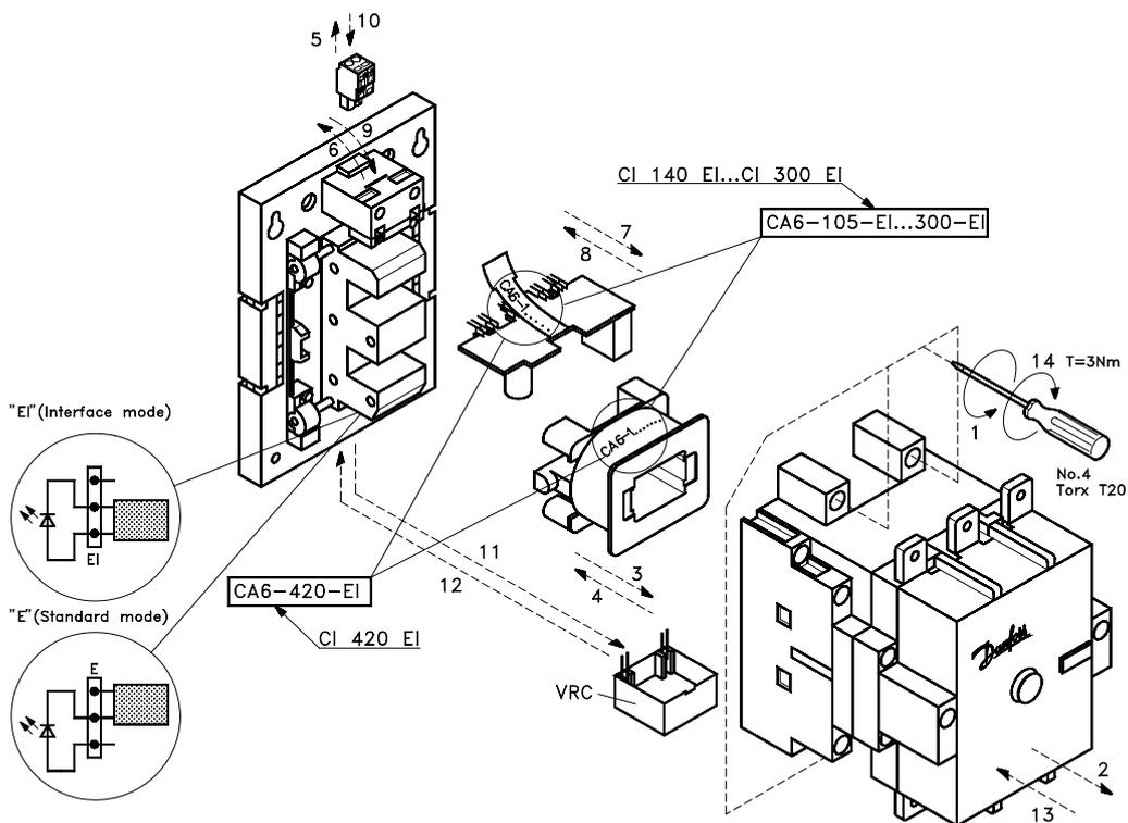
Above is the assembly drawing of contactors with an EI interface. The circles on the left show two alternative control modes of the contactor coil, with PLC or standard, depending on the position of the jumper located under the plug on the bottom of the contactor.
