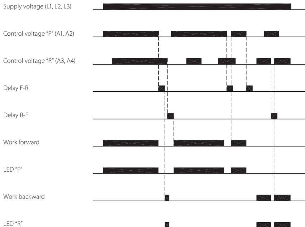
After connecting the power supply, control the A1-A2 circuit so that the motor starts to rotate forward, which is confirmed by the LED light. After supplying the voltage to the A3-A4 control circuit, the motor will start to rotate in the opposite direction, signaling it with the second LED.
