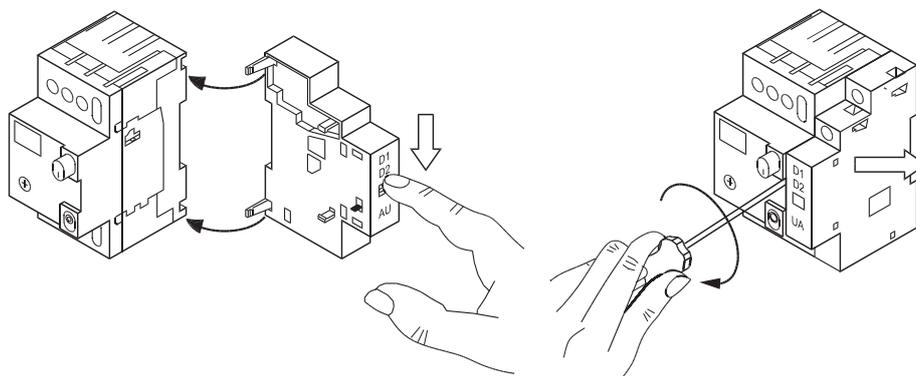
The undervoltage release (UA) is used to remotely switch off the circuit breaker at the moment of power failure in the control circuit (it acts as a safety component).
