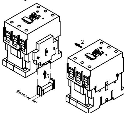
RCD elements RC suppressors are used to reduce the overvoltage in the contactor control circuit.
