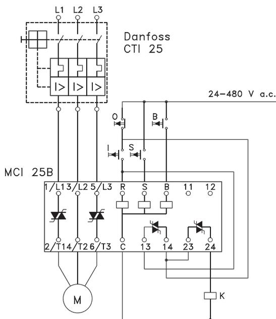
Operation system with external mechanical brake control
