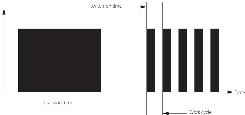
If the contactor is not connected for 100% of the process time, which is the case in most applications, it can carry a load greater than nominal. Load coefficient is the parameter determining acceptable oversizing.
