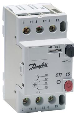
Overload and short circuit protection of three-phase electric motors up to 11 kW. The compact, modular design with a width of 45 mm, equipped with a fast reacting (2 ms) contact system and an advanced arc-quenching chamber, provides short-circuiting capacity up to 65 kA. The mechanical parameters determine the lifetime per 100 000 "on-off" operations at 30 cycles per hour.
