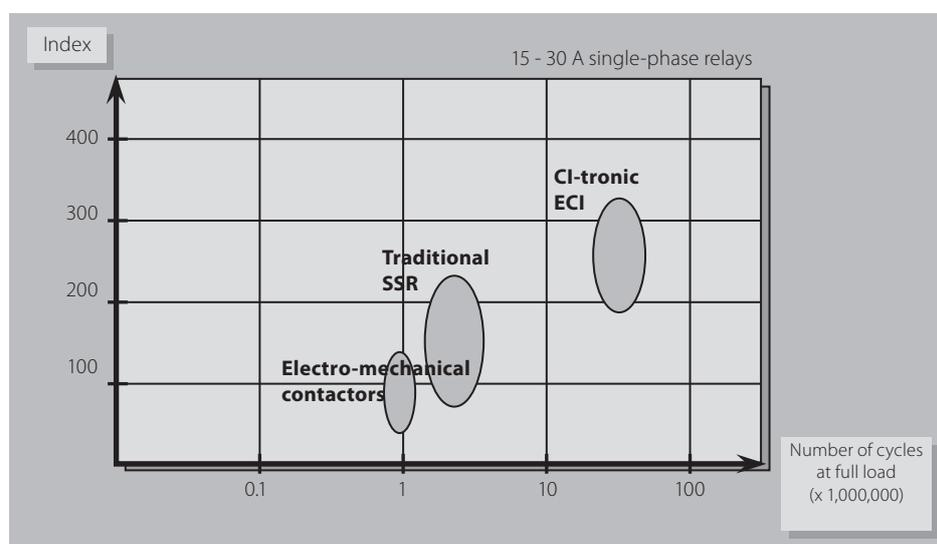
LTE technology enables to achieve an above-average lifespan of up to 50,000,000 cycles, which is on average 10 times more than traditional SSR.
