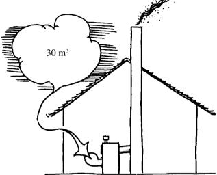
There is a lack of ventilation in the boiler room, i.e. sufficient air is unable to enter the boiler room and the burner fan cannot "breathe". A normal domestic oil-heating plant MUST receive approximately 30 m<sup>3</sup> air per hour. If the fan is prevented from receiving this amount of air, combustion will rise to soot formation.
