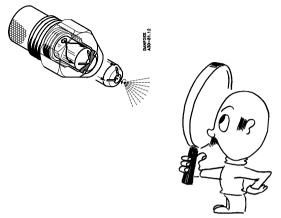
Oil enters through the filter and continues through the bottom screw and its side holes. From there, the oil runs along the side of the cone and into the cone slots.
