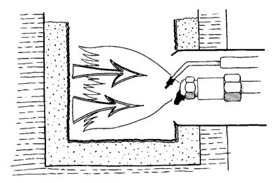
The tendency towards coking is worse on boilers with a heavy fire-brick lining. The reason is that fire-bricks give off strong return radiation which will reach oil particles on the nozzle, ignition electrodes and combustion head during the periods when those parts are not being cooled down by air blast.
