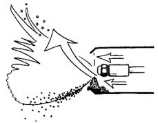
Some of the particles mentioned above continue through the system and lodge in the burner tube causing a poor and uneven oil/air mixture, finally resulting in the flame being lopsided and sooty.
