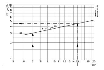
The diagram shows how much oil is discharged from a nozzle marked 3 USgal/h at different atomizing pressures. Worth noticing is the bold line. It starts at the horizontal scale (7 bar) and intersects the inclined line (3 USgal/h line) at 3 USgal/h, illustrating that a 2 USgal/h nozzle does yield precisely that figure when atomizing pressure is 7 bar.
