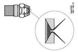
The velocity of the oil film is so great that a "tube" of oil is formed in the nozzle orifice. With the help of that part of the pressure not converted into rotational energy this "oil tube" is forced through the nozzle orifice. On being propelled from the orifice, the "oil tube" is expanded so much that it breaks up into very small oil drops.
