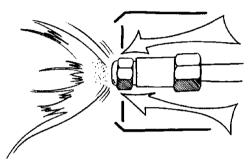
Oil sprayed from a nozzle placed too far back will be caught by the combustion head and may result in oil flooding from the burner tube. Here, it must be pointed out that the higher the fan pressure the plant works with the more accurate must the oil nozzle be located in relation to the burner tube, ignition electrode and combustion head. These remarks principally concern plants which run at 2800 rev/min.
