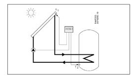
T1: Temperature sensor in solar collector
