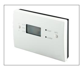
The regulator is used for utility water management in solar heating systems. The solar heat circuit circulation pump is controlled on the basis of the differential temperature between the solar collector and the hot-water tank.
