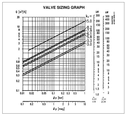
The pressure drop across an H Series valve can be determined from the Kv diagram above.
