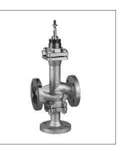
VK 3 valves are a range of 3 port high specification flanged valves for chilled water, LPHW, MPHW, HPHW (low, medium or high pressure hot water) steam and thermo oil applications. The cast iron body with stainless steel plug and seat is suitable for pressures up to 25 bar. These valves may be used with glycol concentrations of up to 50 % making them suitable for ice storage applications.
