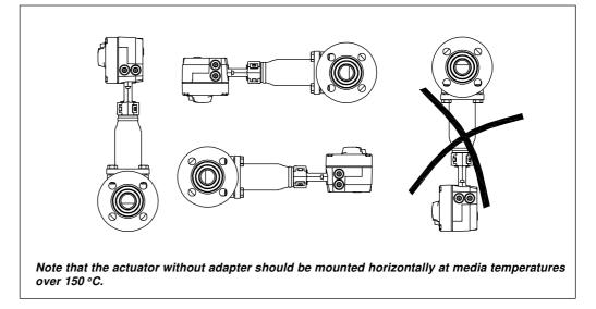
Leave sufficient clearance to facilitate the dismantling of the actuator from the valve body for maintenance purposes.
