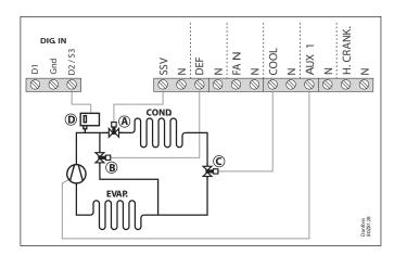
During the process, the liquid solenoid valve (C) and the condenser input valve are closed and the evaporator input valve is opened, forcing hot gas to pass through the latter and melting the ice.
