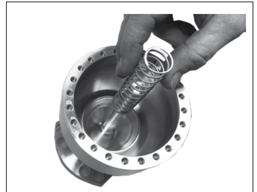
6. Mount the spring on the cone.
