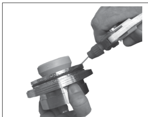
7. Lubricate the O-ring at cover with clean filtered water
