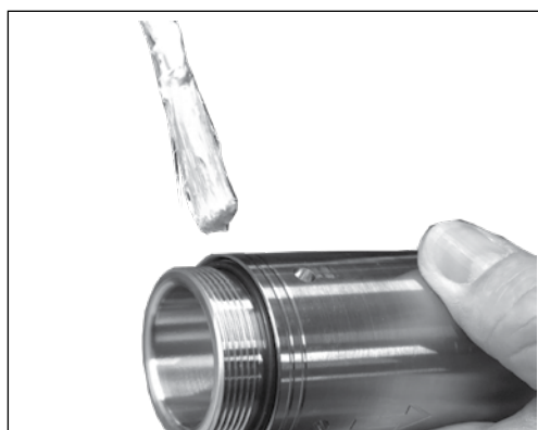
9. Lubricate the threads at the valve end.
