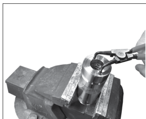
8. Tighten the nut with a snap ring pliers.
