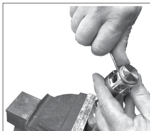
6. Remove the O-ring at the cone with a small screw driver.
