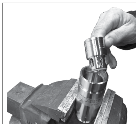
5. Remove the valve cone.
