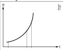
The sensor system contains a fairly large amount of liquid, of which only a small part is brought to vapour form. If the sensor in this type of unit is located warmest in relation to the capillary tube and bellows housing, the ambient temperature has no influence on regulation accuracy.
